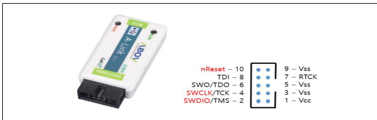
Figure 56. A-Link and Pin Descriptions
