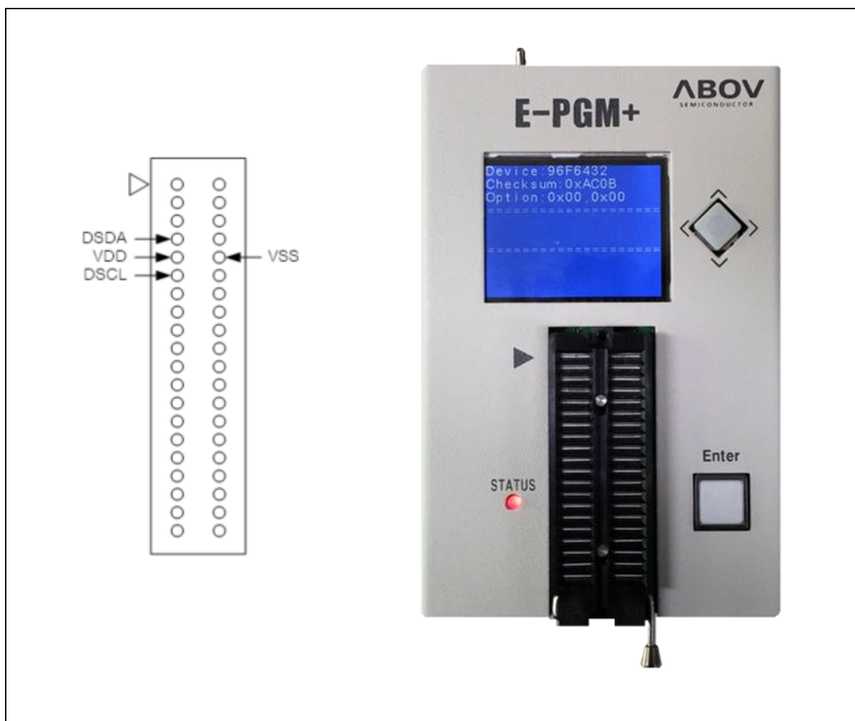
Figure 59. E-PGM+ (Single Writer) and Pin Descriptions
