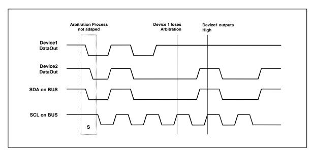
Figure 10 Arbitration Procedure of Two Masters
