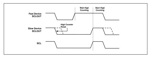
Figure 9 Clock Synchronization during Arbitration Procedure
