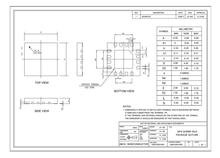
Figure 3 16-pin QFN Package
