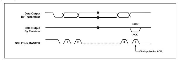
Figure 8 Acknowledge on the I<sup>2</sup>C-Bus
