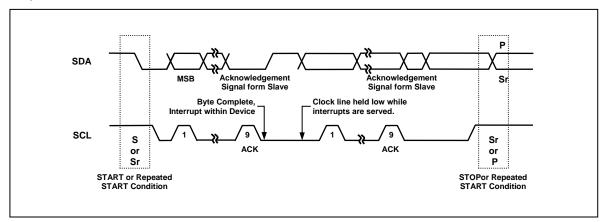
Figure 7 Data Transfer on the I<sup>2</sup>C-Bus
