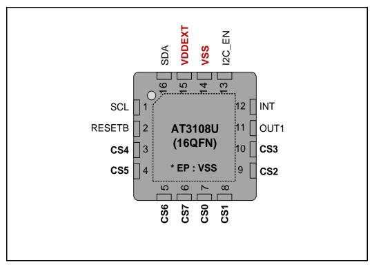
Figure 1 16-QFN Pin Assignment
