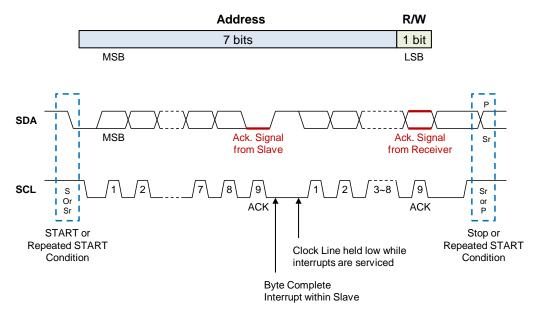
Figure 11 First Byte (Slave Address and R/W)
