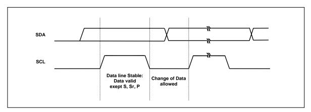
Figure 5 Bit Transfer on the I<sup>2</sup>C-Bus
