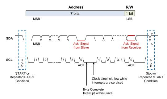
Figure 11 First Byte (Slave Address and R/W)
