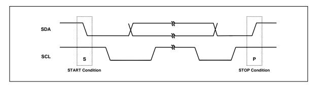
Figure 6 START and STOP Condition
