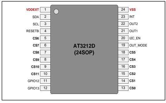
Figure 2 24-SOP Pin Assignment
