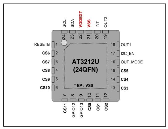
Figure 1 24-QFN Pin Assignment
