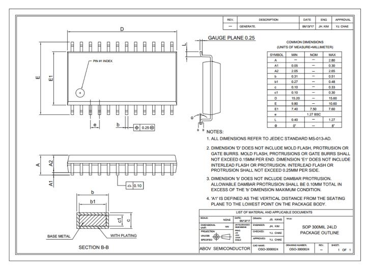
Figure 4 24-pin SOP Package
