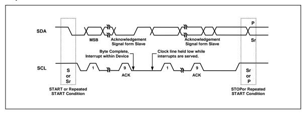
Figure 7 Data Transfer on the I<sup>2</sup>C-Bus
