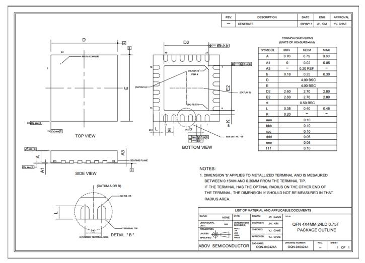
Figure 3 24-pin QFN Package
