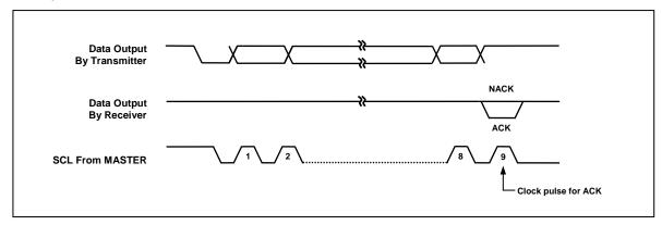
Figure 8 Acknowledge on the I<sup>2</sup>C-Bus
