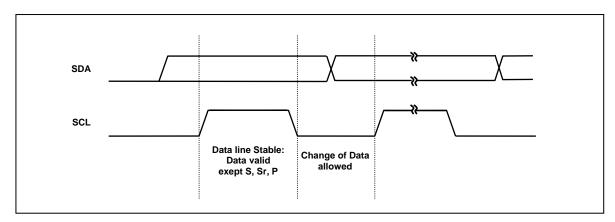
Figure 5 Bit Transfer on the I<sup>2</sup>C-Bus
