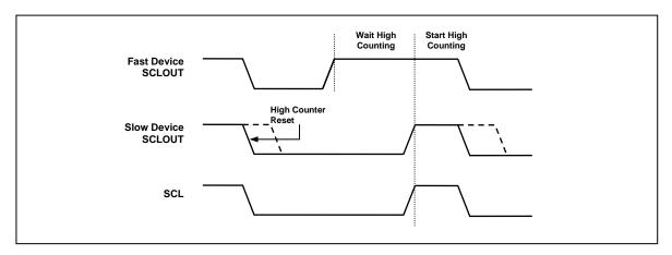
Figure 9 Clock Synchronization during Arbitration Procedure
