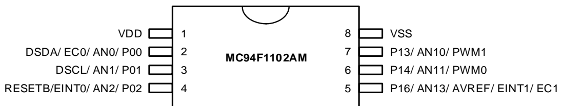
Figure 3.3 MC94F1102AM 8 SOP pin assignment
