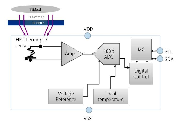
The sensor packaged in a hermetically sealed 4-pin metal can package is RoHS compatible and operates over  $-40 \sim 85^{\circ}$ C temperature range.
